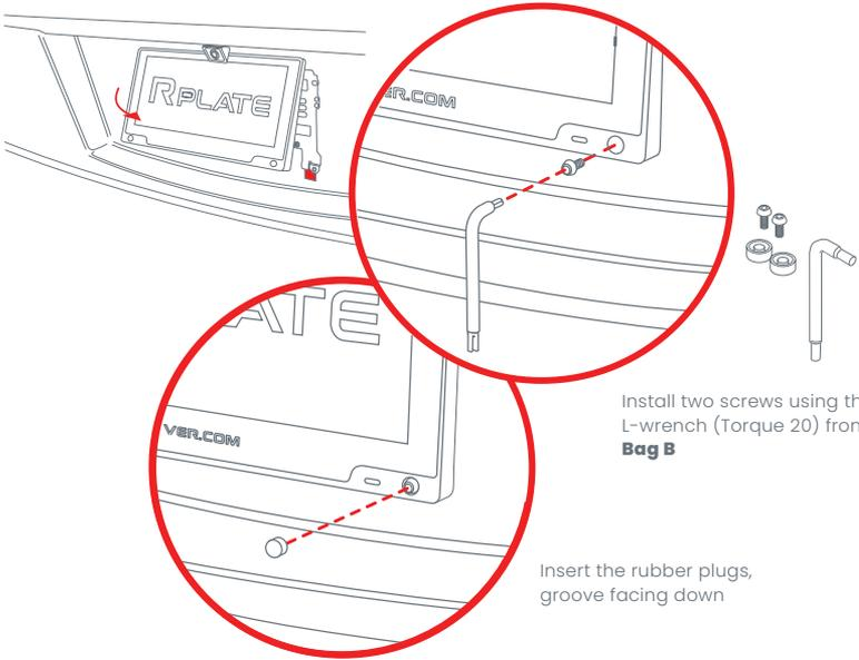
Install two screws using the L-wrench (Torque 20) from **Bag B**
